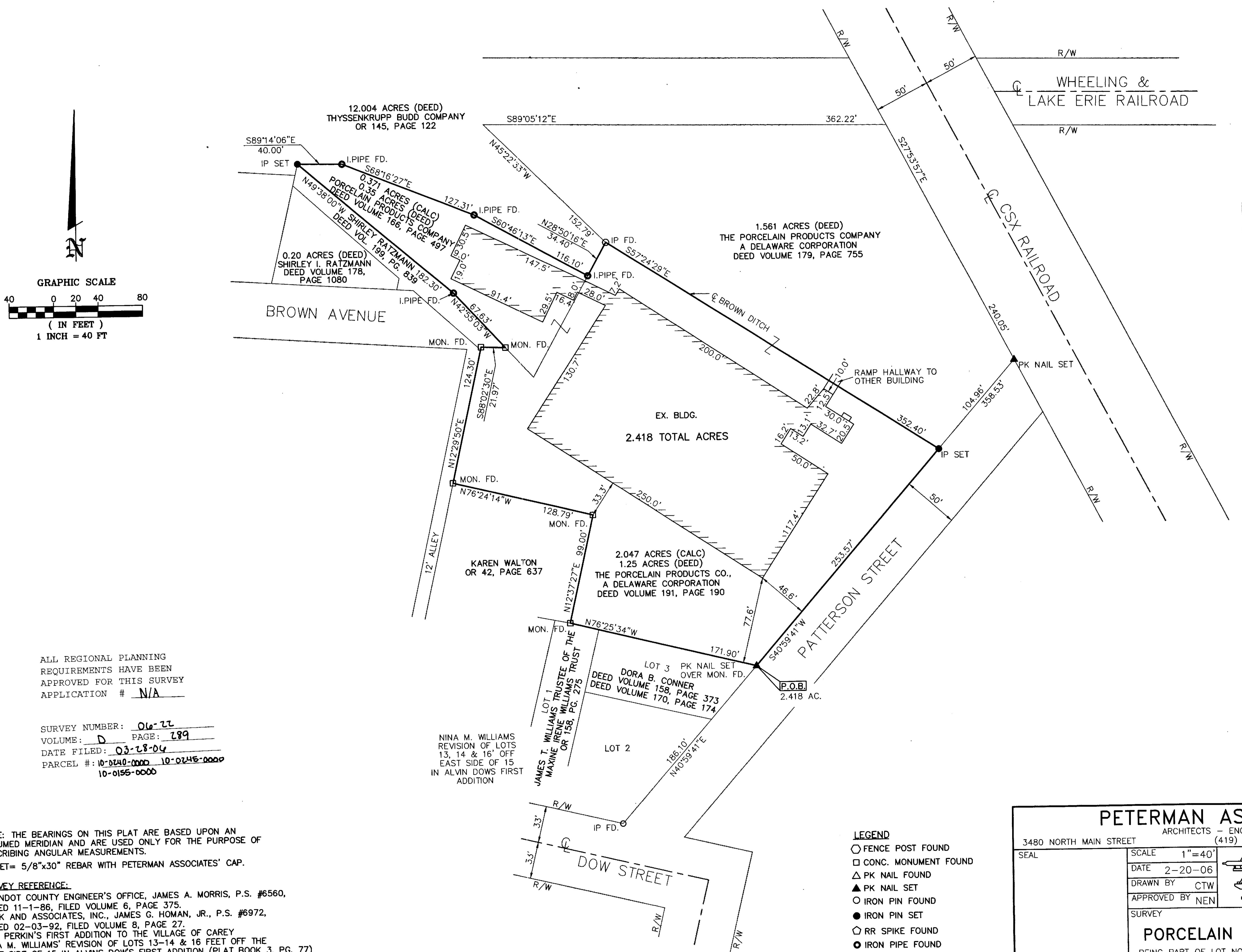
NOTE: THE BEARINGS ON THIS PLAT ARE BASED UPON AN ASSUMED MERIDIAN AND ARE USED ONLY FOR THE PURPOSE OF DESCRIBING ANGULAR MEASUREMENTS.
